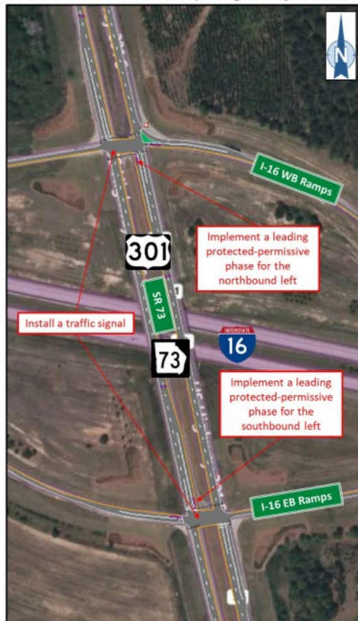
FIGURE 23: RECOMMENDATIONS, SR 73 @ I-16 WB/EB RAMPS
