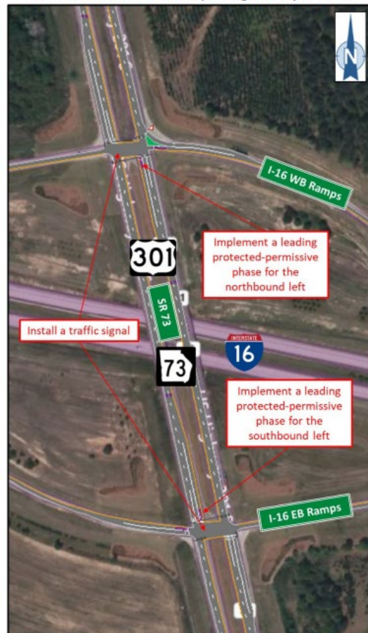
FIGURE 23: RECOMMENDATIONS, SR 73 @ I-16 WB/EB RAMPS
