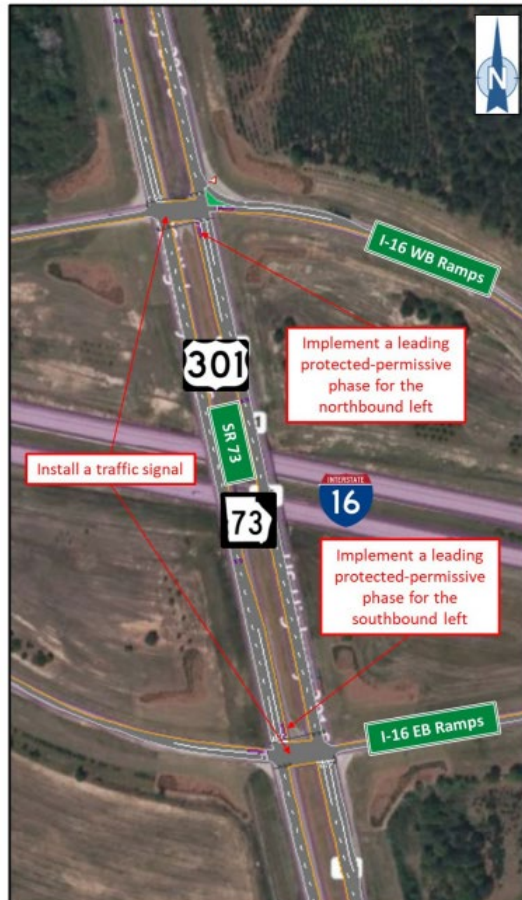
FIGURE 23: RECOMMENDATIONS, SR 73 @ I-16 WB/EB RAMPS
