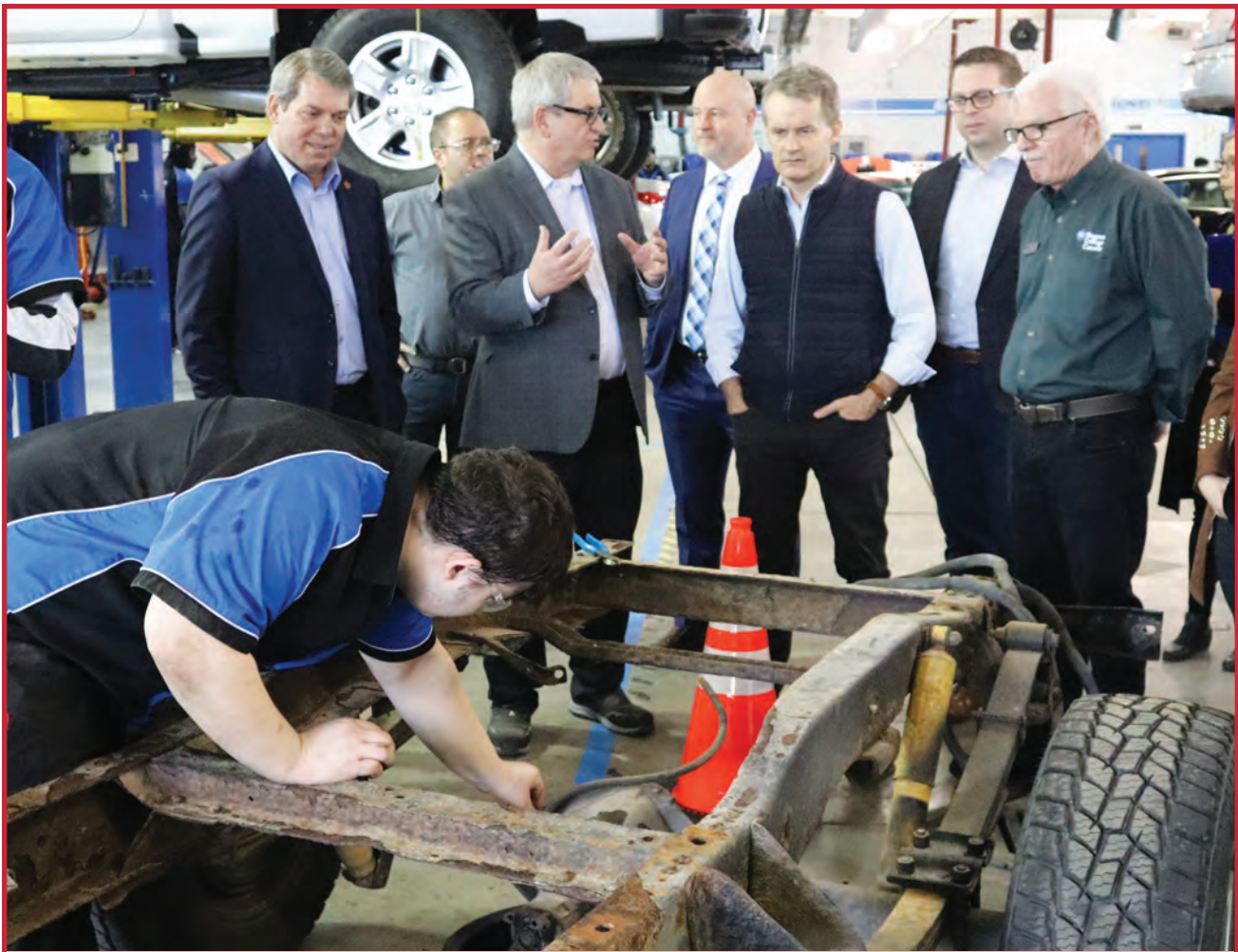
NOTL resident Jonathan Rolph removes a brake line from a chassis to ready it to be retrofitted with an electric battery for conversion into an electric vehicle. He's at Niagara College attending an apprenticeship program. Watching him are Niagara Center MP Vance Badawey, Jeff Murrell (Associate Dean, School of Trades), Niagara College President Sean Kennedy, Federal Minister of Labour Seamus O'Regan, St.Catharines MP Chris Bittle, and Wayne Toth (Automotive Professor/Program Coordinator). O'Regan was at the college to check out the skilled trades and apprenticeship programs. For story see page 7. (Mike Balsom)
